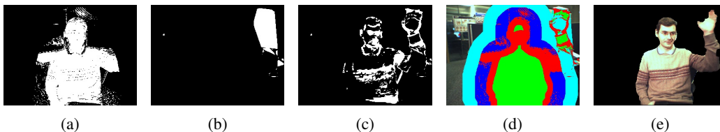
Figure 4: (a) to (e) illustrate the use of (b) motion hulls in addition to (a) colour, face and (c) fused motion edge map to create the final seeds map in (d) which produces the segmentation in (e).
